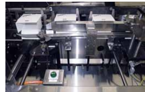
MACHINE INTEGRATION. Integrated servo drives/motors help J&J Ortho improve performance on this cartoning machine.
