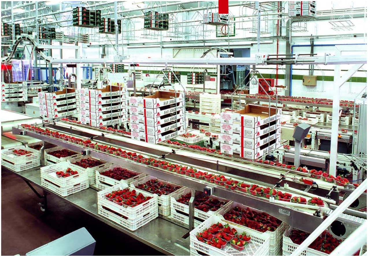
The VarioFlow chain-conveyor system supplies both manual and automatic workstations, acting as a vital link between conveyor belts where the plucked strawberries are supplied in paperboard boxes, and where they are later prepared for shipment in the plastic transport boxes.
