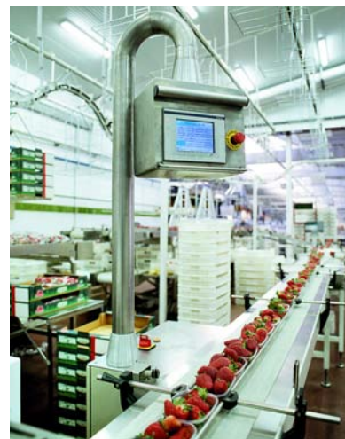
Working in special shifts, the system can deal with up to 1,100 tons of strawberries a day, with the VarioFlow transporting strawberry baskets at up to 50 meters per minute.
